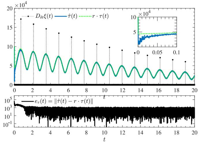
Fig. 7. Noisy experiment (measurement noise standard deviation  $\sigma_{\xi}=0.25$ ). [Above] Norm of the Euler derivative  $D_{\delta t} \xi(t)$ , (dotted black line and circle marker), estimated smoothness bound  $\hat{\tau}(t)$  (blue solid line) and nominal smoothness bound  $\tau(t)$  scaled by the arbitrary constant  $r$ . [Below] smoothness bound approximation error  $e_{\tau}(t)$  (log scale).
