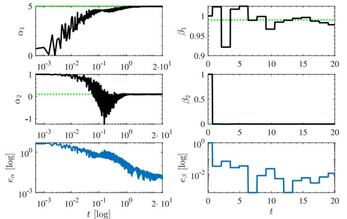
Fig. 8. Noisy experiment (measurement noise standard deviation  $\sigma_{\xi}=0.25$ ): parameters estimation results. [Left] Estimates of the parameters in  $\alpha$  and absolute estimation error  $e_{\alpha}(t) = \|\alpha - \hat{\alpha}(t)\|$  (below). [Right] Estimates of the parameters in  $\beta$  and absolute estimation error  $e_{\beta}(t) = \|\beta - \hat{\beta}(t)\|$  (below).
