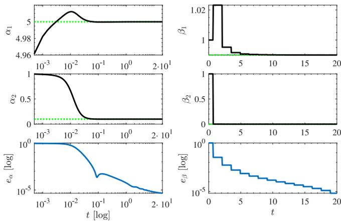
Fig. 6. Nominal experiment (no measurement noise): parameters estimation results. [Left] Estimates of the parameters in  $\alpha$  and absolute estimation error  $e_{\alpha}(t) = \|\alpha - \hat{\alpha}(t)\|$  (below). [Right] Estimates of the parameters in  $\beta$  and absolute estimation error  $e_{\beta}(t) = \|\beta - \hat{\beta}(t)\|$  (below).
