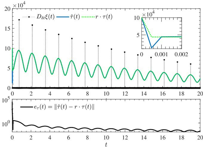
Fig. 5. Nominal experiment (no measurement noise). [Above] Norm of the Euler derivative  $D_{\delta t} \xi(t)$ , (dotted black line and circle marker), estimated smoothness bound  $\hat{\tau}(t)$  (blue solid line) and nominal smoothness bound  $\tau(t)$  scaled by the arbitrary constant  $r$ . [Below] smoothness bound approximation error  $e_{\tau}(t)$  (log scale).
