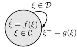
Fig. 1. Hybrid automata: Conceptual representation of the hybrid system  $\mathcal{H}$  characterized by a single flow map  $f$  and one jump map  $g$ . Only one state and one reset branch are needed to picture the behaviour of the system.
