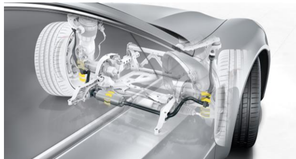
Fig. 1. Electromechanical active roll stabilization at the front axle of a vehicle.
