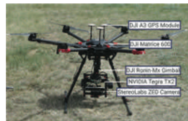
Fig. 1. Our experimental setup for Visual Teach & Repeat (VT&R) on a multirotor UAV.
