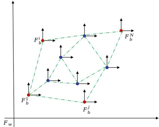
Fig. 1. Sensing and communication topology of robots formation
