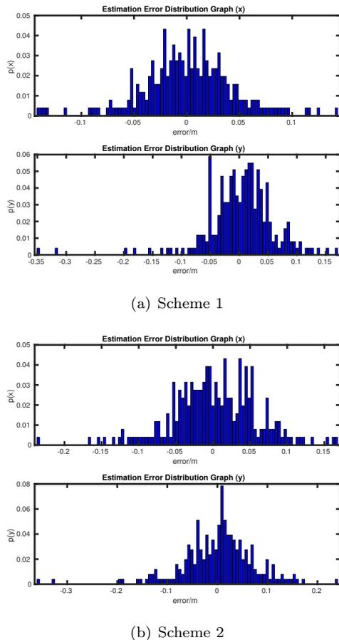
Fig. 5. The statistics of random error for relative navigation system ( Fig (a) and (b) represent the random error of estimation based on accurate ONS and inaccurate GPS respectively. )
