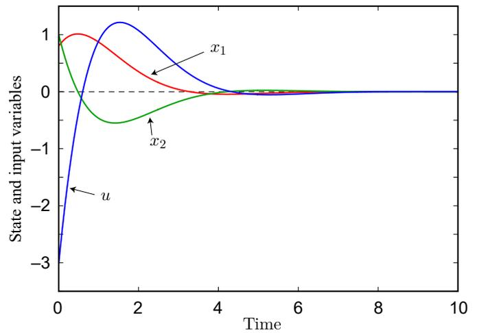
Fig. 6. Time responses of state and input variables of simulation result for LQ regulator.
