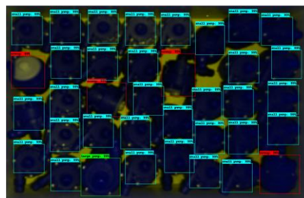
Fig. 6. Detected pumps and misaligned objects (Faster R-CNN with Resnet 101)
