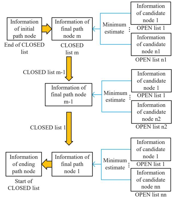
Fig. 1. Flow diagram of traditional A\* algorithm
