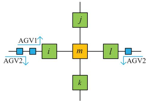
Fig. 6. Schematic diagram of AGV conflicts in path network
