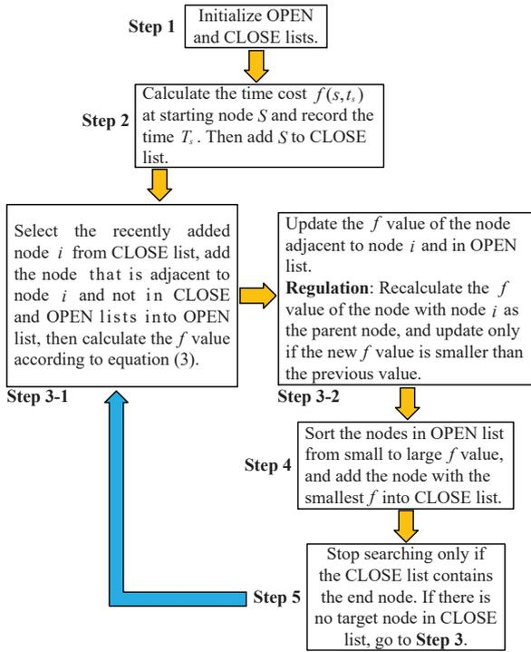
Fig. 4. Flow diagram of improved heuristic algorithm
