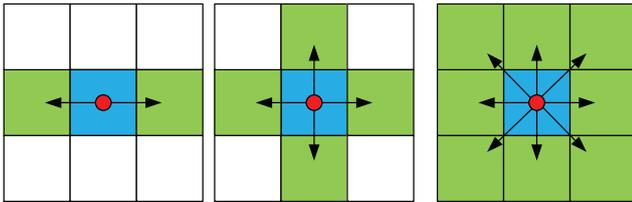
Fig. 3. Schematic diagram of 2-direction, 4-direction and 8-direction motion in path network
