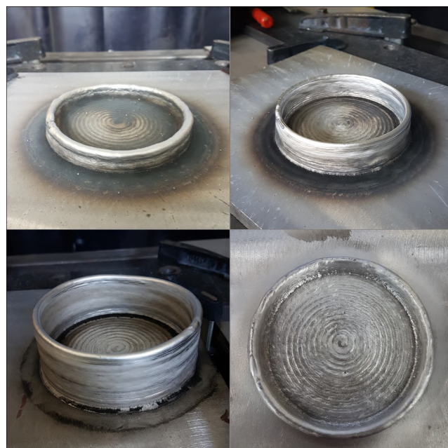
Fig. 5. Set-based control: The structures built in the first three tests, and close-up of the bottom.
