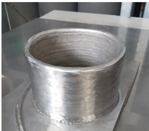
Fig. 4. Vertical welding gun: Cylindrical structure built with fixed, vertical orientation of the welding gun, with continuous height increase like that shown in Figure 2.
