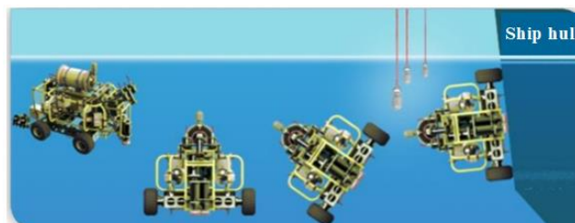
Fig. 1 Docking process of ROV Iznos
