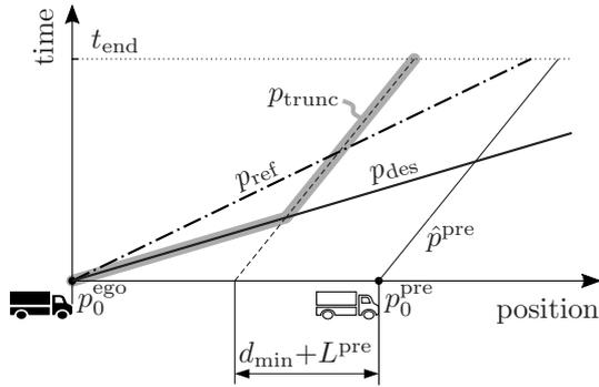
Fig. 2. Determining the scalar reference velocity  $v_{\text{ref}}$  from the predicted position trajectory at desired velocity  $v_{\text{des}}$ , clipped by predicted predecessor interference.
