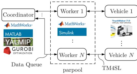
Fig. 3. Validation via vehicle dynamics co-simulation.
