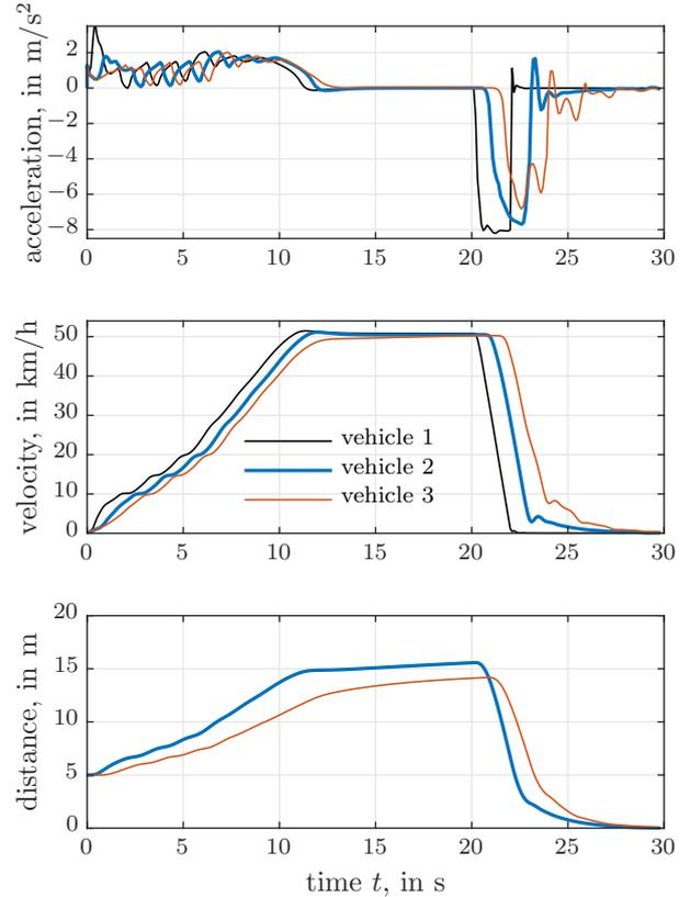
Fig. 5. Validation on dry road:  $\hat{\mu} = 0.8$ ,  $\hat{\mu}^{\text{pre}} = 1.2 \mu^{\text{ego}}$
