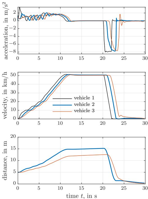
Fig. 6. Validation on dry road:  $\hat{\mu} = 0.8$ ,  $\hat{\mu}^{\text{pre}} = 1.0$   $\hat{\mu}^{\text{ego}}$
