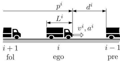
Fig. 1. Geometric specifications of a vehicle with a follower and a predecessor.
