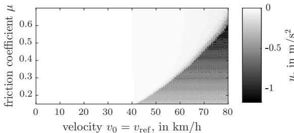
Fig. 4. Control law evaluated at  $u_{-1} = 0$ ,  $d_b = 50 \text{ m}$  over  $\mu$  and velocity
