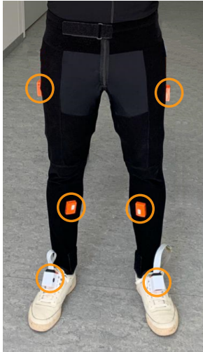
Fig. 3. Subject wearing IMUs (orange), pressure insoles and sensor brackets (white) laced to the shoes.
