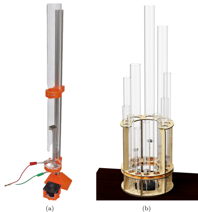
Fig. 8. (a) Prototype platform with single Rijke tube and (b) full 11-tube Rijke organ instrument
