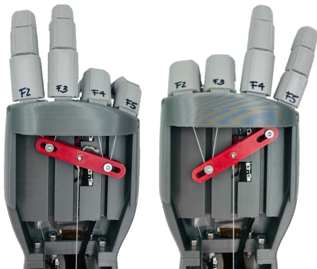
Fig. 6. Rocker (red bar) of the differential mechanism. Different positions of the rocker according to the resistance on the finger.
