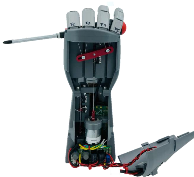
Fig. 4. Cylindrical grasp. Holding a screwdriver with TSA. Forearm and hand chamber are opened.
