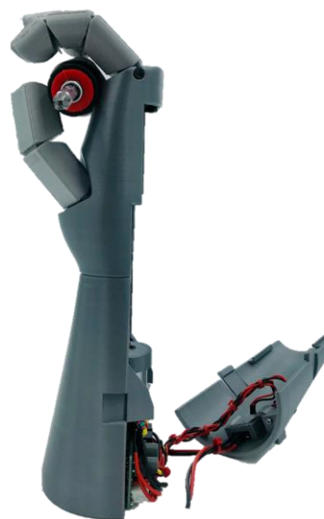
Fig. 5. Cylindrical grasp (side view). Holding a screwdriver with TSA. Forearm and hand chamber are opened.
