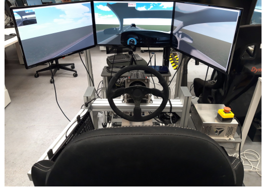
Fig. 4. DiL automated driving simulator
