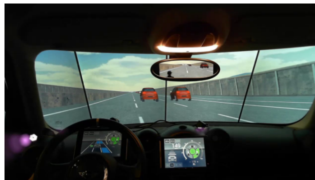
Fig. 2. Driving simulator showing a lane change manoeuvre
