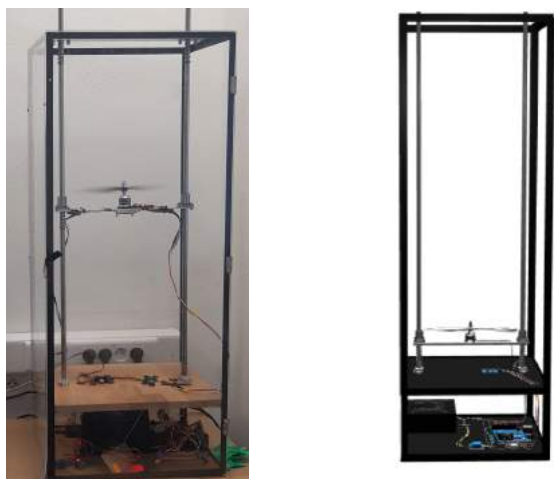
Fig. 3. Real towercopter plant and the 3D model created in Blender rendered by babylon.js
