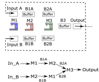
Fig. 4. Production process of a manufacturing system: Logical layout and process plan.
