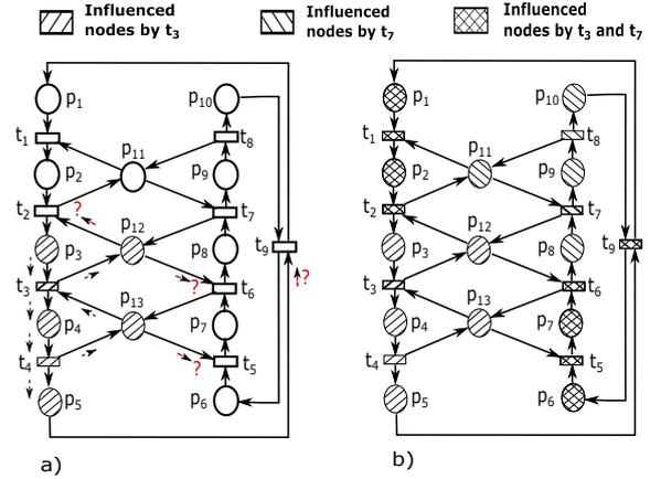
Fig. 2. On influence in TCPNs: a) Influenced nodes by the control action of  $t_3$ . For some configurations, it is blocked at join transitions. b) Influenced nodes when  $T_c = \{t_3, t_7\}$ . In this case  $P_I = P$  and  $T_I = T$ .
