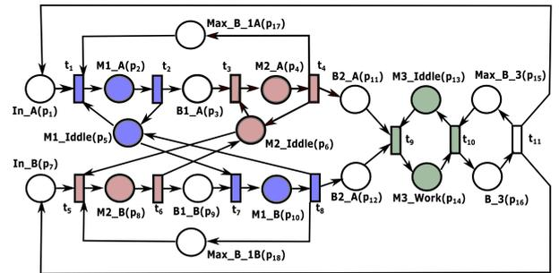
Fig. 5. *TCPN* that models the flexible system in Fig. 4. It has 216 possible configurations.
