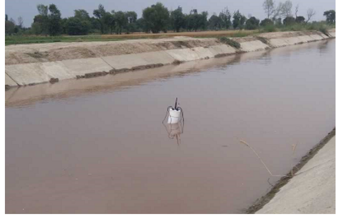
Fig. 1. The Lagrangian sensor equipped with GPS floating in a canal.
