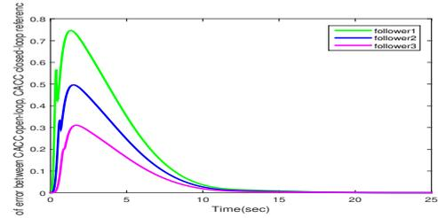
Fig. 4. Norm of error between CACC open-loop, CACC closed-loop reference model for uncertain vehicles in the platoon.
