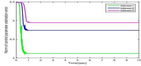
Fig. 3. Norm of controller parameter estimation-error  $\tilde{K}(t)$  for uncertain vehicles in the platoon.
