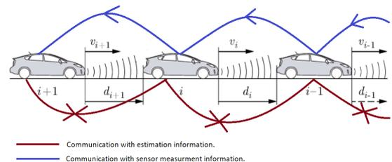
Fig. 1. CACC based homogeneous vehicle platoon.
