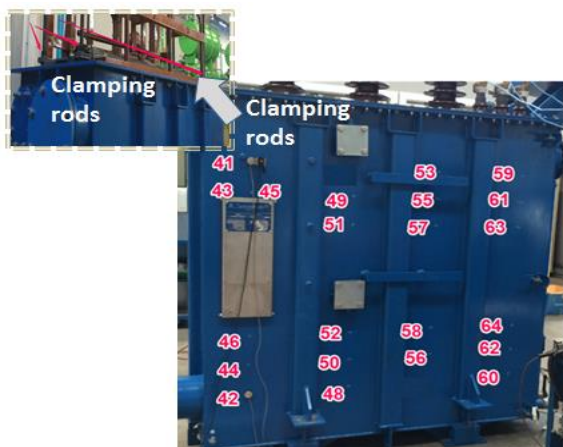
Fig. 1. The 750kVA test transformer. Insets: a detail of the looseness of winding clamping structure (left) and of measurement points (right).
