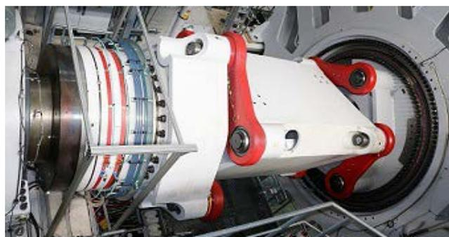
Fig. 3. Torque limiter, flexible coupling, moment bearing
