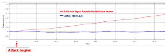
Fig. 17. Ramp-function Bias Injection Attack: The behavior of the slow attack.
