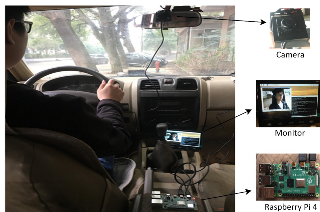
Fig. 9. Raspberry Pi 4 with driver fatigue detection model in the real driving environment.
