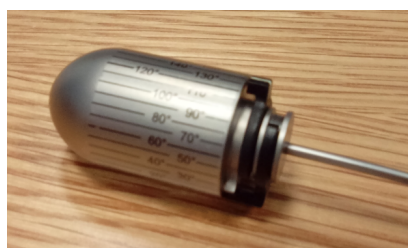
Fig. 3. Measurement device for the accurate and easy measurement of the angles of valve commissure positions on the aorta wall during the open heart surgery.
