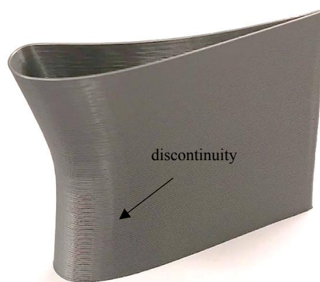
Fig. 4. Printing results of the aerofoil fabricated based on a STL file generated by 0.1 mm tolerance for the chordal error.
