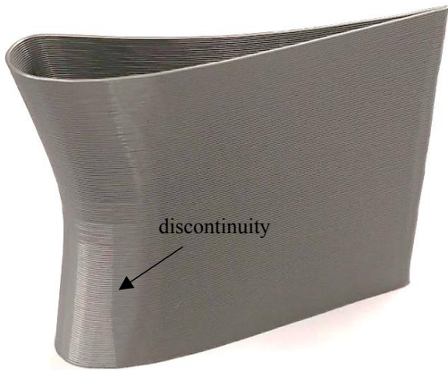
Fig. 5. Printing results of the aerofoil fabricated based on a STL file generated by 0.2 mm tolerance for the chordal error.
