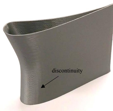
Fig. 3. Printing results of the aerofoil fabricated based on a STL file generated by 0.05 mm tolerance for the chordal error.
