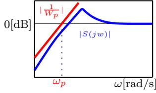
Fig. 4. Figure of constraint for sensitivity function
