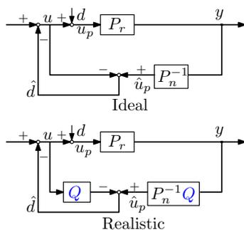
Fig. 1. Block diagram of ideal and realistic disturbance observers
