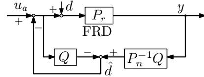
Fig. 2. Block diagram of disturbance observer system
