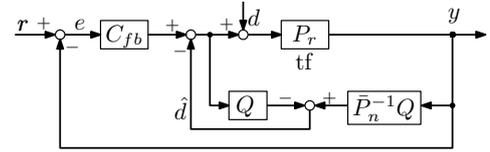
Fig. 11. Block diagram of disturbance compensation based on DOB
