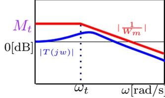
Fig. 5. Figure of constraint for complementary sensitivity function
