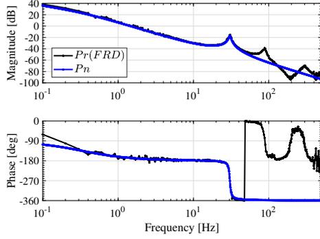
Fig. 8. Bode plots of plant FRD ( $P_r$  (FRD)) and nominal plant ( $P_n$ )
