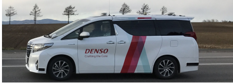
Fig. 4. Experimental vehicle equipped with high-precision GNSS, LiDAR, radar, and cameras.
