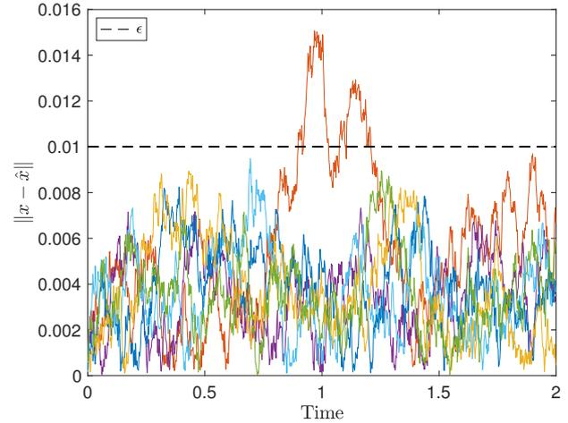
Fig. 1. A few realizations of the errors between concrete state trajectories and estimated trajectories.
