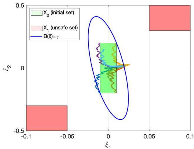
Fig. 2. A few realizations of the closed-loop trajectories using controller (5.2). The blue ellipsoid shows the  $\gamma$ -level set of  $B$ , defined as  $\{\hat{x} \in X \mid B(\hat{x}) = \gamma\}$ .
