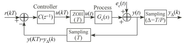
Fig. 3. Process model in closed-loop system
