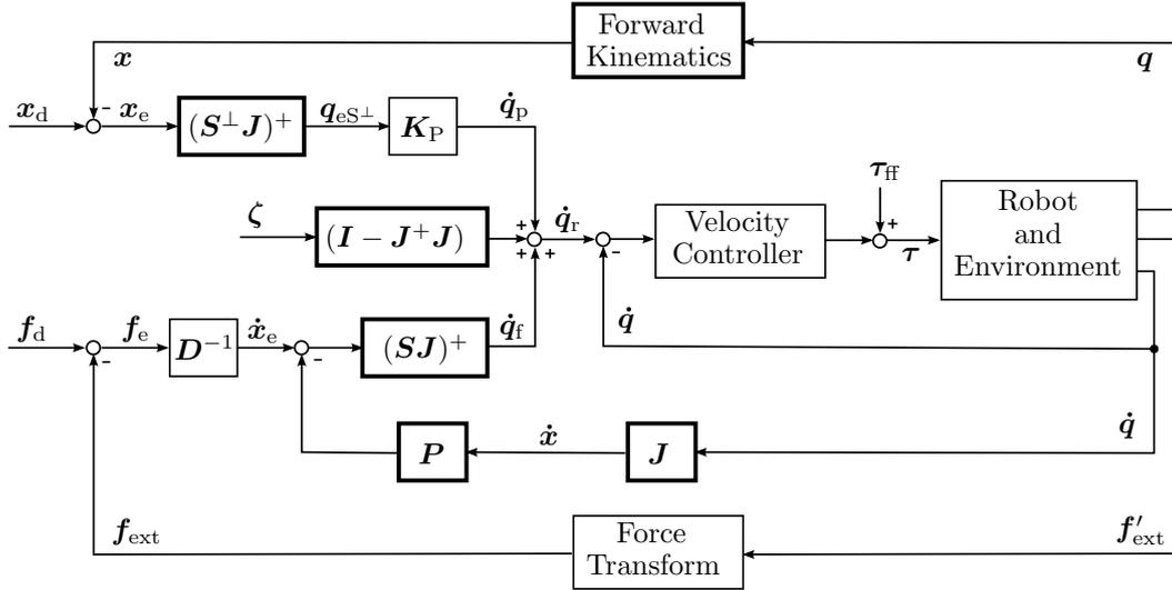
Fig. 1. Structure of the proposed velocity-based hybrid force/motion control scheme, where the modifications to the original structure are highlighted by bold blocks, i.e., the nonlinear proportional controllers  $(\mathbf{S}\mathbf{J}(\mathbf{q}))^+\mathbf{D}^{-1}$  and  $\mathbf{K}_P(\mathbf{S}^\perp\mathbf{J}(\mathbf{q}))^+$ , the additional Cartesian velocity feedback  $\mathbf{P}\mathbf{J}$  and a null space input.
