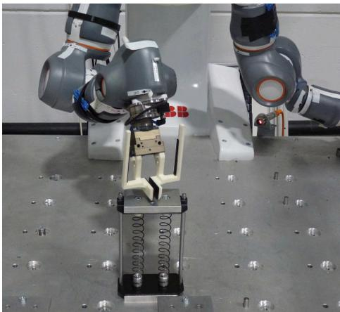
Fig. 2. Experimental setup with end-effector motion in the Cartesian  $z$ -direction hitting an unexpected environment with stiffness  $K_e = 1000 \text{ N m}^{-1}$ .
