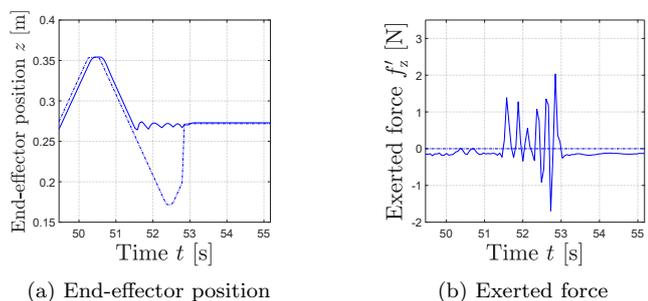
Fig. 4. Position and force measurements in setup 1 using the trial and error method ( $D_z = 5 \text{ N s m}^{-1}$ ) showing an unstable bouncing interaction with the environment (dashed lines show references).
