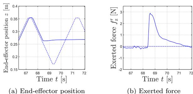
Fig. 5. Position and force measurements in setup 1 using the generalized eigenvalue approach ( $\delta_{\Lambda_T, z} = 1$ ) showing a critically damped interaction with a minimum of exerted force (dashed lines show references).
