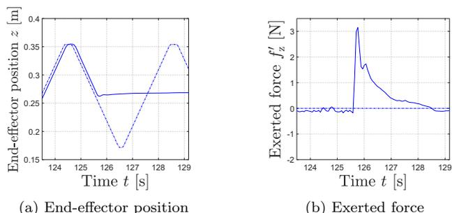
Fig. 3. Position and force measurements in setup 1 using the trial and error method ( $D_z = 40 \text{ N s m}^{-1}$ ) showing a damped interaction behavior with risk to oscillations (dashed lines show references).
