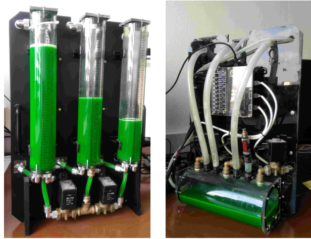
Fig. 1. Three-tank laboratory system - front and back view
