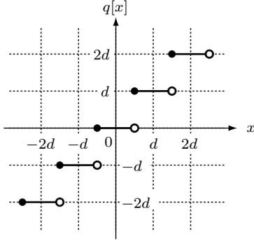
Fig. 2. Static uniform quantizer with quantization interval  $d$
