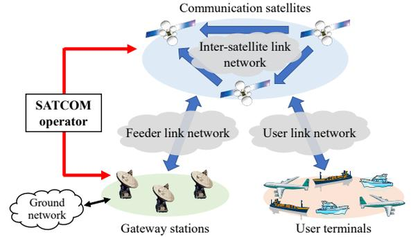
Fig. 1. Schematic of the large-scale SATCOM systems.
