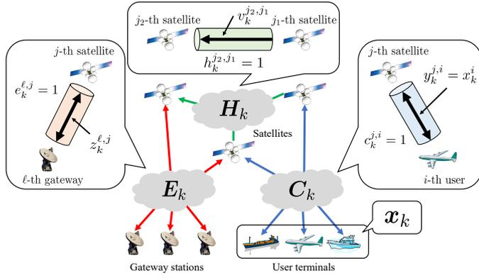
Fig. 2. Notations of the resource allocation and network structure in large-scale SATCOM systems.
