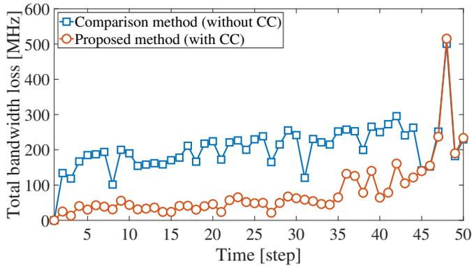
Fig. 5. Total bandwidth loss of the proposed method with  $\Delta^i = 0.1$  (red line) and the comparison method (blue line).
