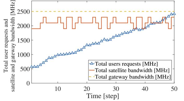
Fig. 3. Time-varying total user requests (blue line), total satellite bandwidth (red line), and total gateway bandwidth (dashed yellow line).
