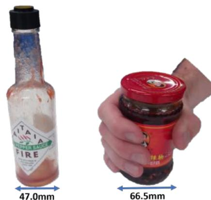
Fig. 2. Objects, sauce (left) and chilli (right), with diameters 47mm and 66mm respectively
