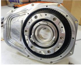
Fig. 4. Traction module view without external cover
