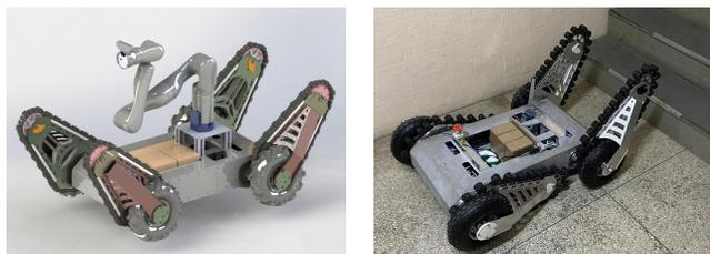
Fig. 1. ROSI - a tracked/wheeled mobile robot
