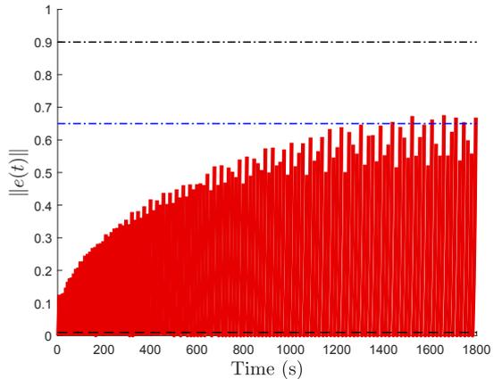
Fig. 2. Evolution of error  $\|e(t)\|$  when  $x(t) \notin \mathcal{F}$ . The black (top) dashed line represents the maximum allowable error  $e_M$  and the blue (bottom) dashed line represents the extremum point of the output function that the ESC minimizes. The error increases to the extremum point while remaining bounded by  $e_M$  for all time.
