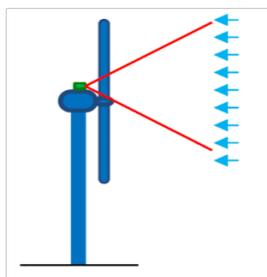
by applying a feed-forward action in response to incoming changes in wind, such as gusts. The availability of a predictive measurement of the main disturbances also enables the use of Model Predictive Control algorithms. Yaw control can be improved if the wind direction measured by the lidar is more accurate than that measured
