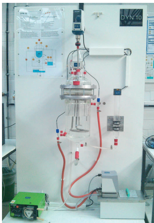
Figure 10.1: Experimental setup of the thermal part of the CSTR located at TU Dortmund.
