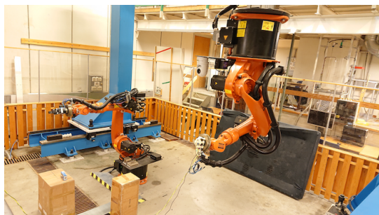
Fig. 1. Thrivaldi is a floor-mounted and a gantry-mounted KR16, currently with a pneumatic SCHUNK gripper (RH9010), and an IMU attached, respectively.
