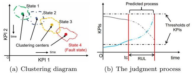
Fig. 3. Threshold-based degradation state estimation
