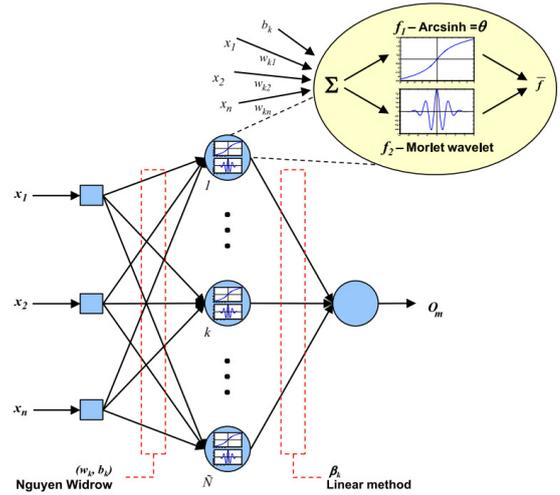
Fig. 1. Structure of SW-ELM (Javed et al. (2014))
