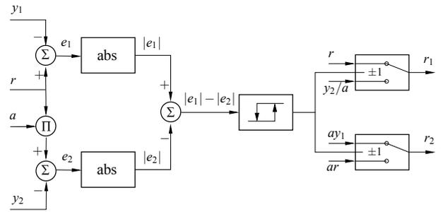
Fig. 2. Block diagram presentation of the Tracking Ratio Station.
