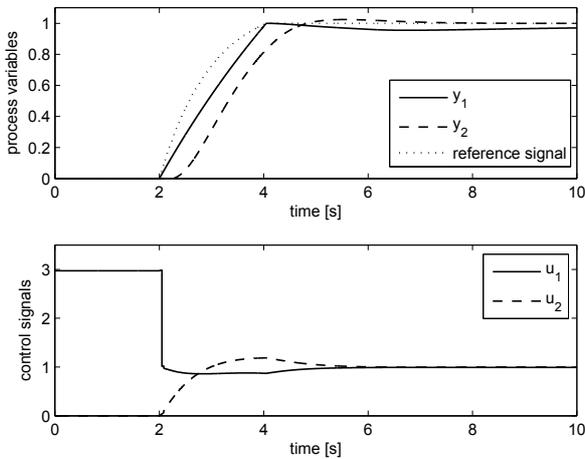
Fig. 5. Results related to Example 1 with the two-state feedforward action and  $u_{max} = 3$ .
