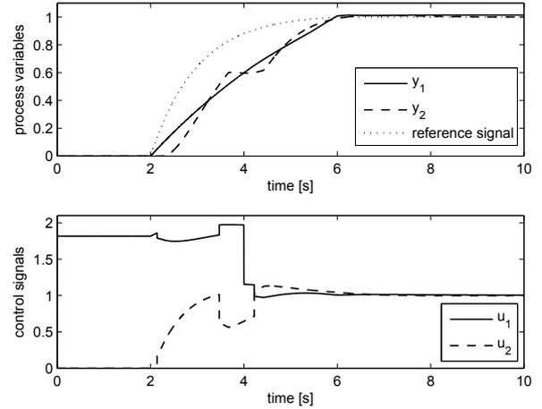
Fig. 3. Results related to Example 1 with the two-state feedforward action and  $u_{max} = 2$ .
