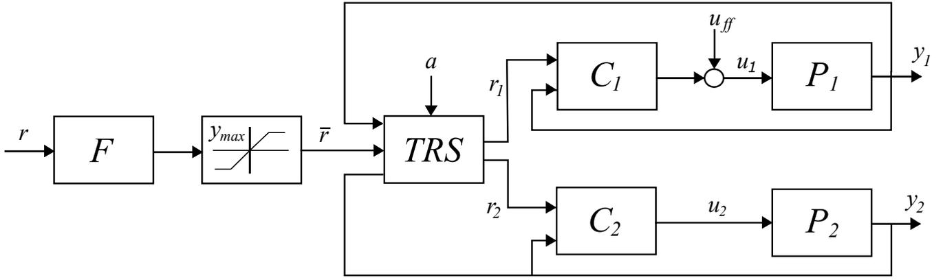
Fig. 1. Control scheme of the proposed ratio controller.
