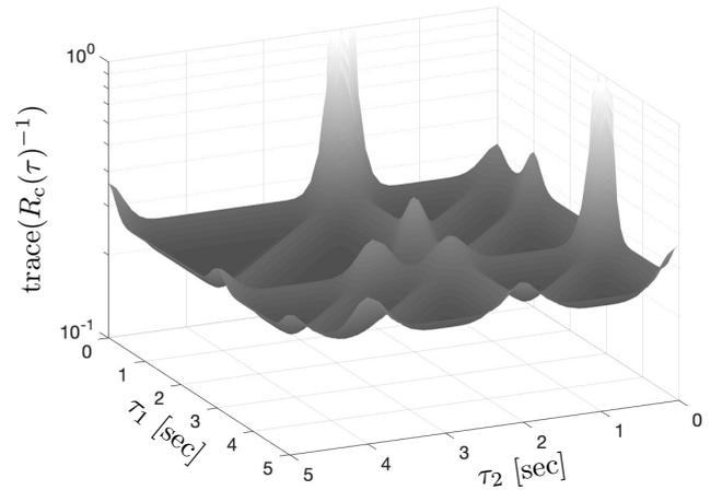
Fig. 2. Lower bound on the estimation error of any non-intrusive load monitoring algorithm in Theorem 1 [top] and Corollary 2 [bottom] versus scheduling delays of the first two loads.
