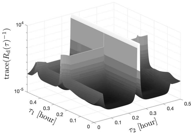
Fig. 4. Lower bound on the estimation error of any non-intrusive load monitoring algorithm in Theorem 1 versus scheduling delays of the first two loads.
