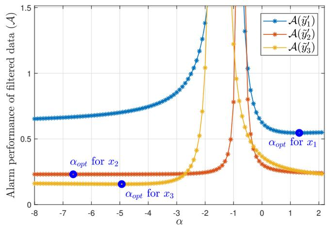
Fig. 3. Analytically evaluated optimal  $\alpha$  (using the equation in (27)) and simulation result for various choices of  $\alpha$  with  $N = 3$ .
