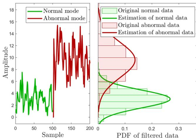
Fig. 5. Time trend and histogram of  $y_2$  (filtered version of  $x_2$  according to the scenario 1 with  $N = 3$ ).
