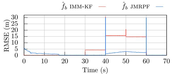
(b) RMSE barometer fault estimate.
