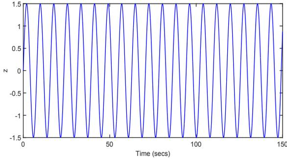
Fig. 4. Common forcing disturbance  $z = A \sin \omega t$  for  $A = 1.5$ ,  $\omega = 0.8$ .
