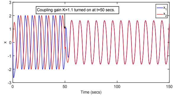
Fig. 5. Synchronization of two Van der Pol oscillators for  $\mu=1$ , coupled to a common forcing with coupling gain  $K=1.1$  introduced at  $t=50$  secs.
