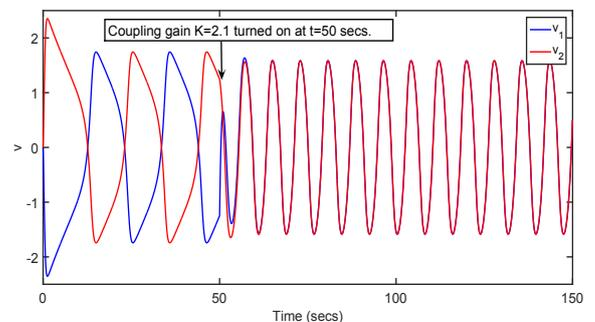
Fig. 8. Synchronization of two Fitzhugh Nagumo oscillators for  $c=1$ , coupled diffusively to a common forcing disturbance with coupling gain  $K=2.1$  introduced at  $t=50$  secs.
