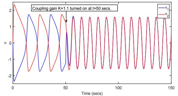
Fig. 7. Synchronization of two Fitzhugh Nagumo oscillators for  $c=1$ , coupled diffusively to a common forcing disturbance with coupling gain  $K=1.1$  introduced at  $t=50$  secs.
