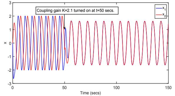
Fig. 6. Synchronization of two Van der Pol oscillators for  $\mu=1$ , coupled to a common forcing with coupling gain  $K=2.1$  introduced at  $t=50$  secs.
