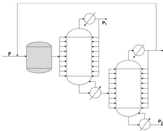
Fig. 2. Conventional reactor-distillation-recycle process
