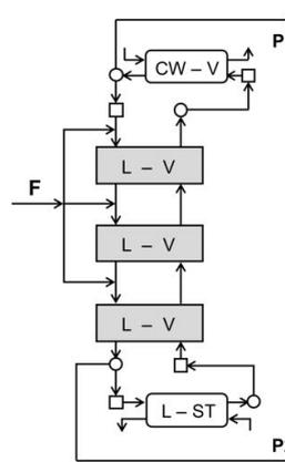
Fig. 4. GMF representation – Reactive distillation.
