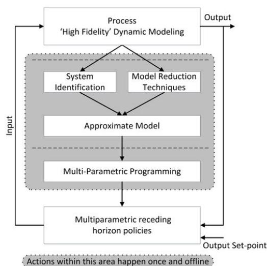
Fig. 7. The PAROC framework (adapted from Pistikopoulos et al. (2015)).
