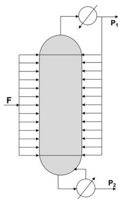
Fig. 1. Intensified reactive distillation process.
