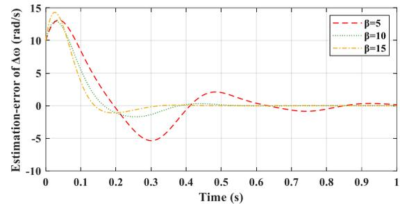
Figure 4. Estimation error of rotor angular velocity difference for the considered values of  $\beta$ .
