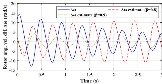
Figure 6. Actual and estimated states of rotor angular velocity difference for boundary  $\beta$ .
