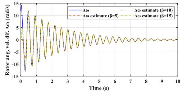
Figure 2. Actual and estimated states of rotor angular velocity difference for various values of  $\beta$ .
