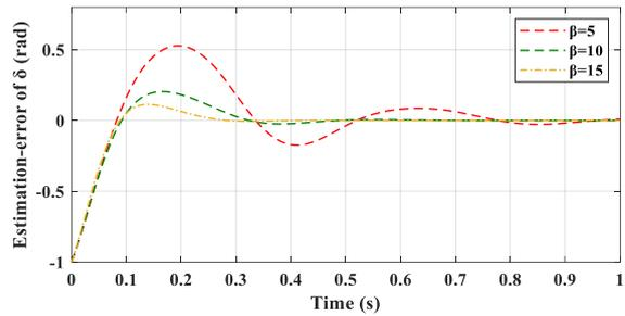
Figure 3. Estimation error of rotor angle for the considered values of  $\beta$ .
