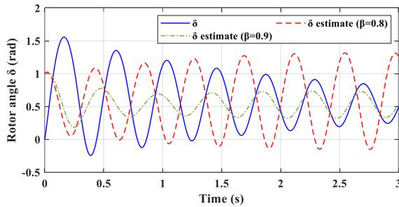
Figure 5. Actual and estimated states of rotor angle for boundary  $\beta$ .
