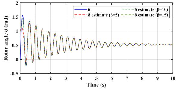
Figure 1. Actual and estimated states of rotor angle for various values of  $\beta$ .
