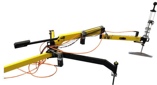
Fig. 1. Granular-fill Insulation Distributing Robot with SCARA-like configuration. An actuated arm with an end-effector tool is used to distribute the filling material in order to smooth the to be processed surface.
