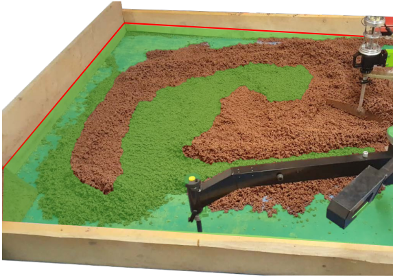
Fig. 3. A laser level is used to highlight the desired floor height (red). Knowing the orientation of the camera, an artificial plane is placed in the point cloud to point out the areas with a too high (brown) or insufficient (green) amount of material.
