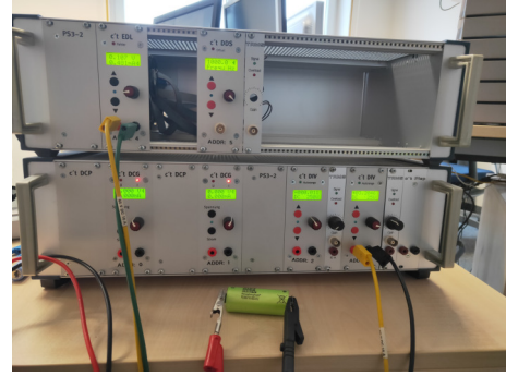
Fig. 2. Instrumental set-up for voltage measurement.
