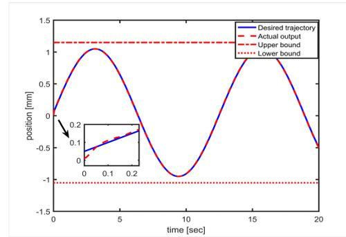
Fig. 3. Actual outputs and reference trajectory under fixed-time state feedback control based RBFNN.
