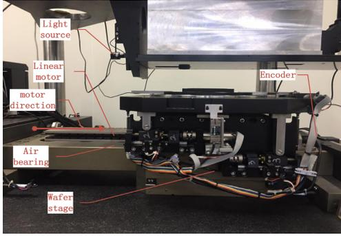
Fig. 1. The lithography machine system.
