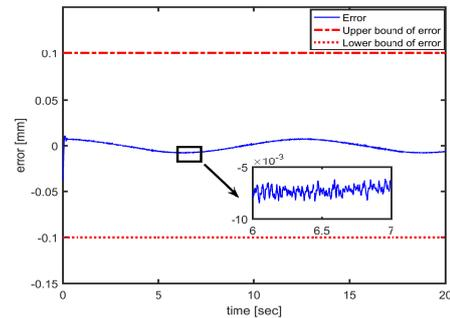
Fig. 4. Tracking errors  $e_1 = x_1 - y_d$  under fixed-time state feedback control based RBFNN.
