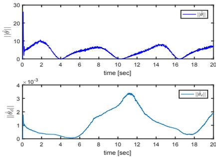
Fig. 6. Euclidean norm  $\|\hat{\theta}\|$ ,  $\|\hat{\theta}_d\|$  under fixed-time state feedback control based RBFNN.
